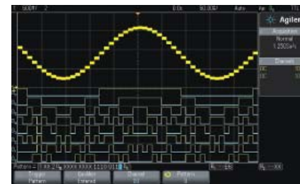
3000 X-Series MSO adds 16 integrated digital channels for extra triggering and analysis; DSO models are customer-upgradable to MSO models
