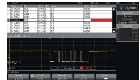
500 CAN serial packets over 9 seconds, captured at a high sample rate, using the 3000 X-Series's segmented memory
